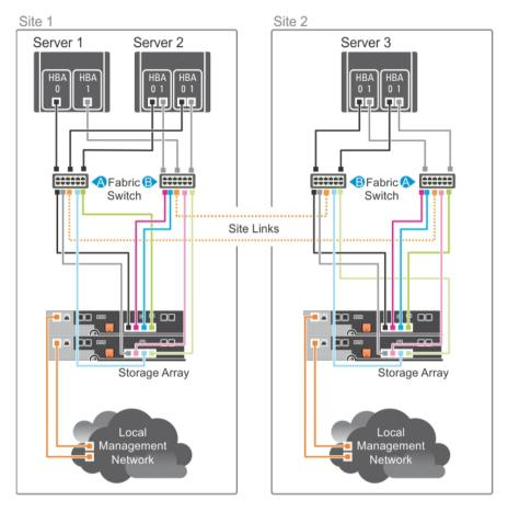
Figure 3. Remote Replication Cabling
